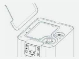
You will see the white top of the MAXI filter cartridge towards the back of your BIBO with a handle protruding from it. Turn the handle firmly anti-clockwise until the filter cartridge releases, then pull it up and out of the BIBO.
