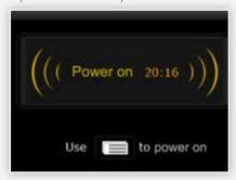
Touch the key to confirm you want it to turn on. When BIBO switches back on again from the power on/off mode, the hot tank will take approximately 5 minutes to heat back up to the maximum temperature and the cold tank will take approximately 15 minutes to chill back down to the minimum temperature.
